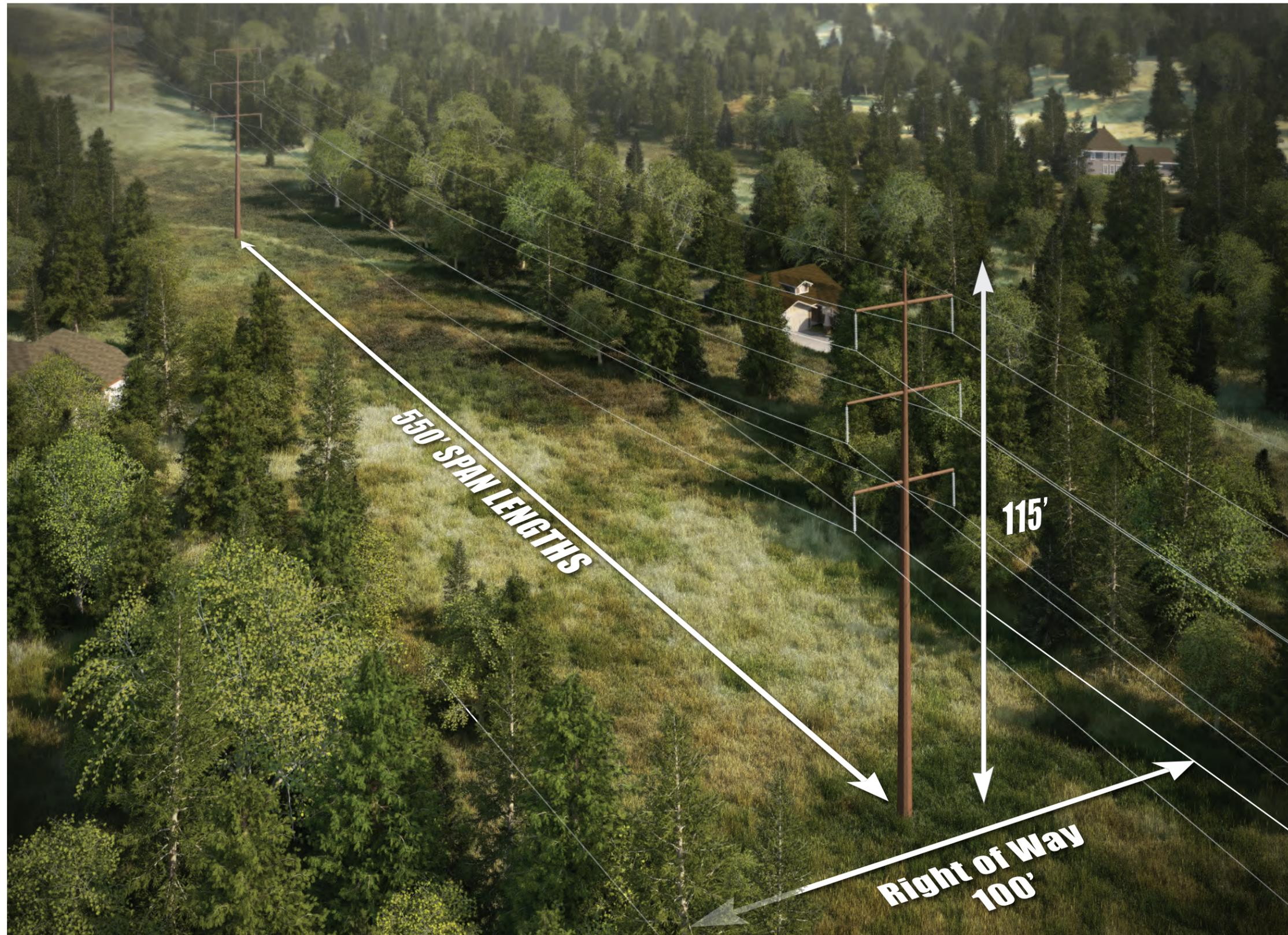
Note: Span lengths and heights shown are typical and may vary due to localized site conditions and engineering requirements.
