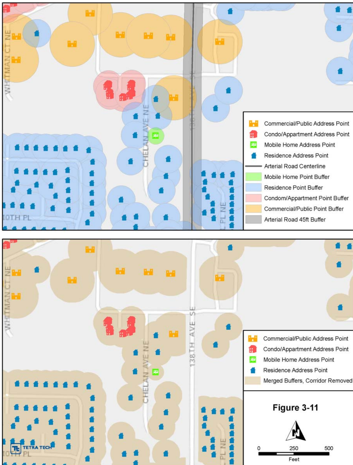
Figure 3-11. Structure Buffer Process
