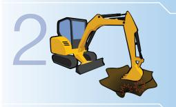
CONSTRUCTION MISHAPS - Power interruptions can occur when a construction-equipment operator accidentally digs into an underground cable.
