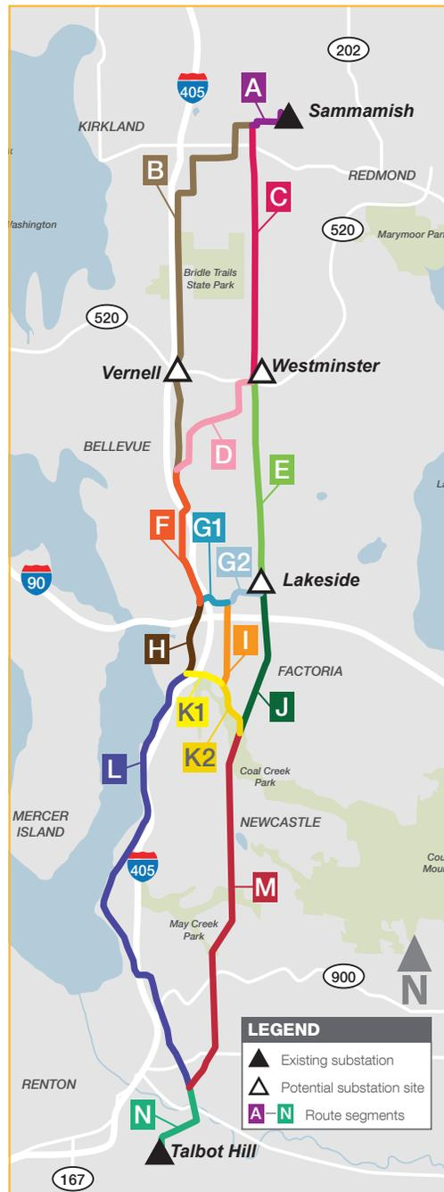
*Route options will be configured to go from segment A to segment N and connect with one of the potential substation sites.*
