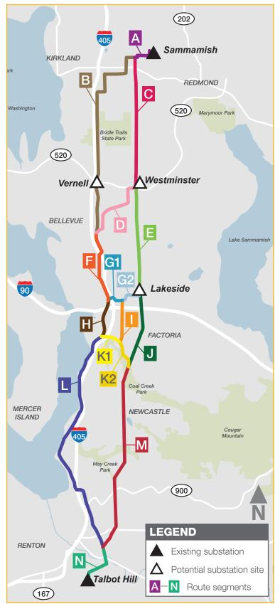
Route options will be configured to go from segment A to segment N and connect with one of the potential substation sites. Visit pse.com/energizeeastside to view the project route segments.
