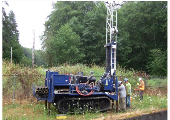
While equipment can vary by property, geotechnical boring is typically completed by a truck- or track-mounted drill rig.
