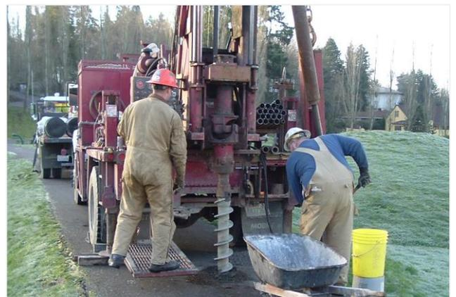
An example of a truck-mounted drill rig.
